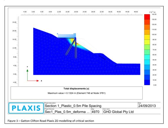
The PLAXIS 2D modelling raised some interesting questions during the design process in relation to the geometry of the micropiles and their interaction with the capping beam which are not addressed in the FHWA design process.
