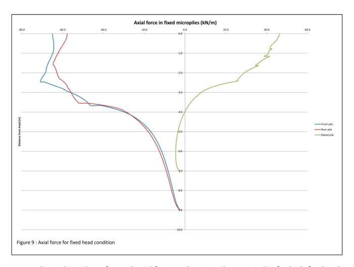
From the analysis, the unfactored axial force in the micropiles was similar for both fixed and pinned head conditions with the pinned head condition producing a slightly higher force per micropile.
