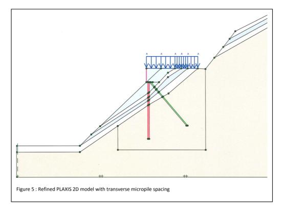
With the transverse micropile spacing included in the model, the ultimate condition under full Q100 flood level and high water table reduced from 55mm in the initial model to 3.5mm in the refined model.
