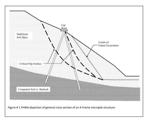
The FHWA design procedure focuses on solving the geotechnical aspects of the slope stability problem. Although it gives some guidance on the potential size of the capping beam, its scope is limited to determining the required shear resistance to achieve a suitable factor of safety for a deep slip and leaves the structural design of the capping beam mostly up to the structural designer.
