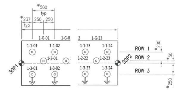
Figure 7: Final micropile layout
